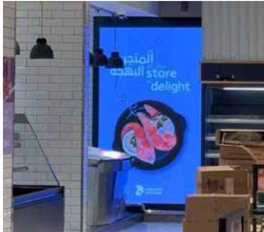
P1.8 INDOOR LED SCREEN Screen size : 269 x 160 cm Module size : 32 x 16 cm
