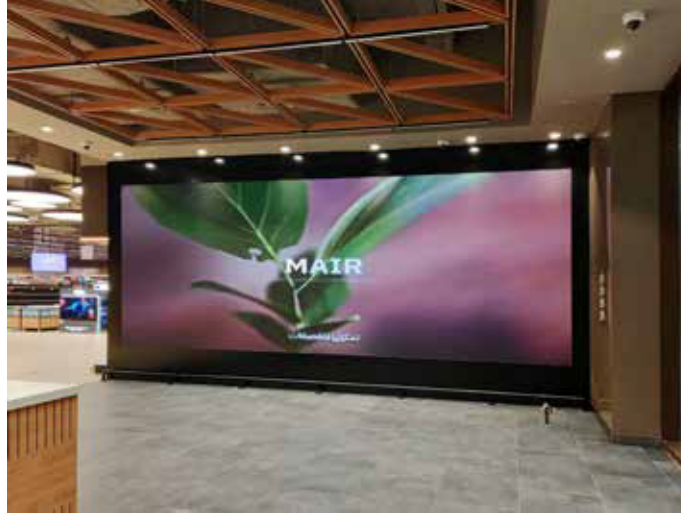
P1.8 INDOOR LED SCREEN Screen size : 756 x 375 cm Module size : 32 x 16 cm
