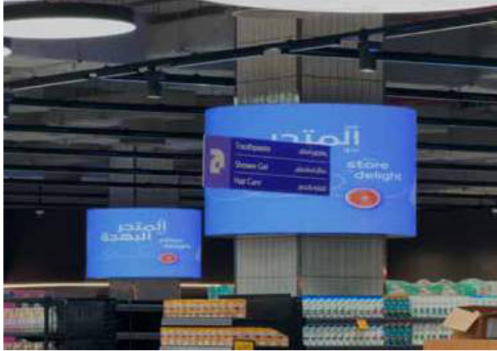
P1.8 INDOOR LED SCREEN Screen size : 512 x 96 cm Module size : 32 x 16 cm
