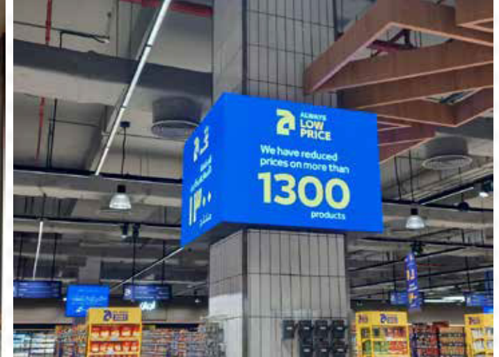
P1.8 INDOOR LED SCREEN Screen size : 128 x 96 cm Module size : 32 x 16 cm
